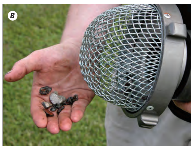
Figure S8.7. (A) Flowing hydrant with Plant PRO HFD hydrant flow tester (pitot tube with wire-cage diffuser), and (B) debris found in diffuser after conducting C-factor test, Hadnot Point–Holcomb Boulevard study area, U.S. Marine Corps Base Camp Lejeune, North Carolina, August 25, 2004.
