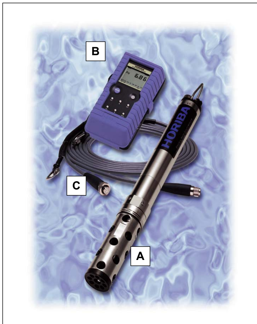
Figure 16. Photograph showing: (A) HORIBA W-21XD single probe water-quality measurement logger, (B) control unit for downloading data from logger, and (C) cable to connect control unit to probe.
