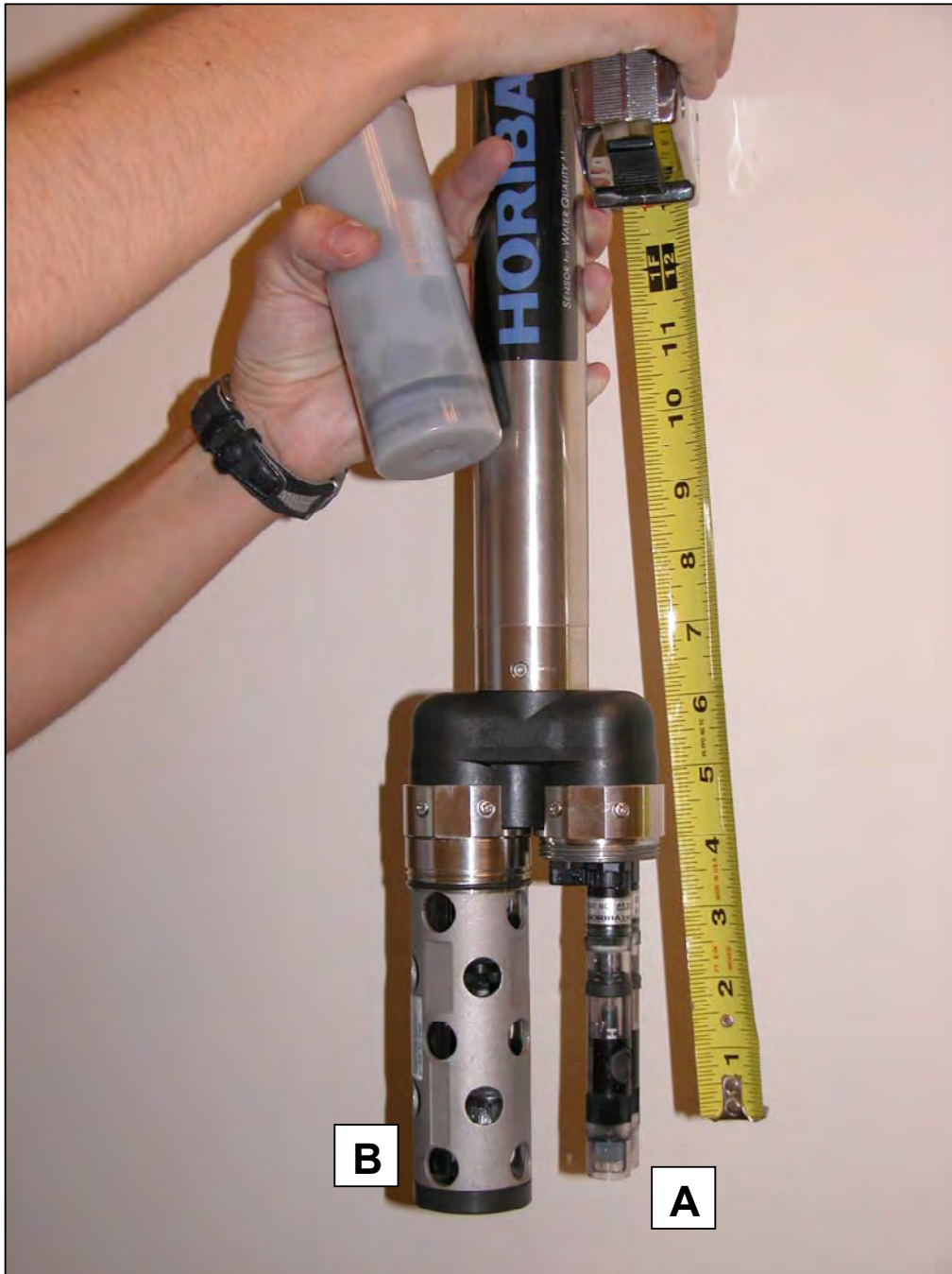
Figure 10. Photograph showing HORIBA W-23XD dual probe ion detector with: (A) fluoride and chloride sensors, and (B) pH, temperature, and conductivity sensors (located inside metal housing).
