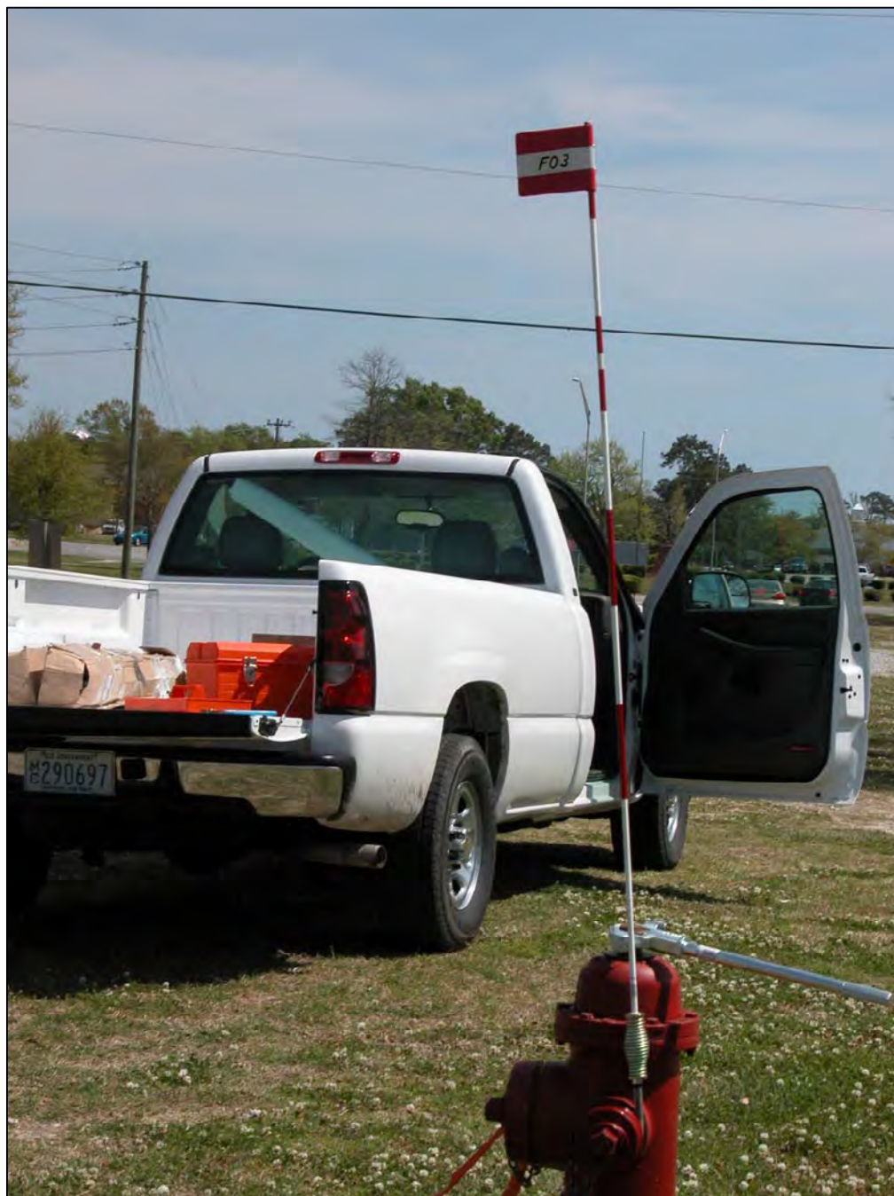
Figure 6. Photograph showing sampling hydrant F03 marker flag mounted on 5-foot fiberglass pole (refer to Plate 1 and Appendix F for hydrant location).
