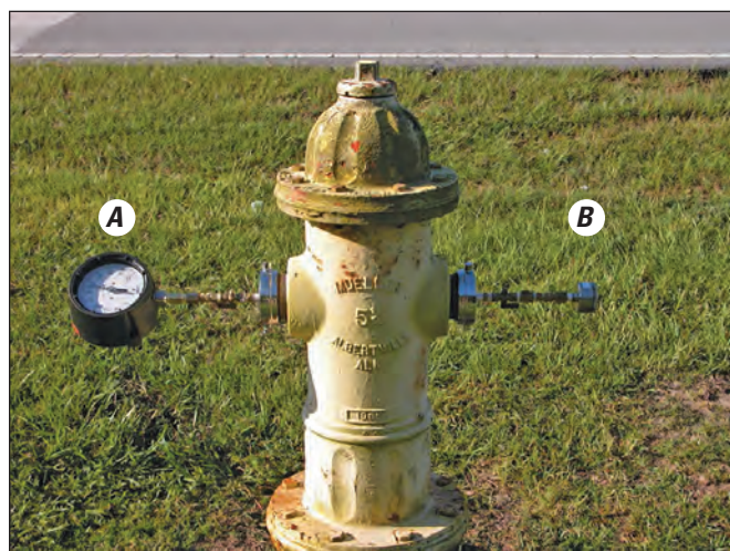
Figure S8.6. C-factor test hydrant equipped with (A) WIKA 4-inch, 0–100 psi, manual reading gauge, and (B) Dixon PR300, 0–300 psi, pressure data logger gauge (recording time set to 1-minute intervals on data logger), Hadnot Point–Holcomb Boulevard study area, U.S. Marine Corps Base Camp Lejeune, North Carolina, August 25, 2004. [psi, pounds per square inch]
